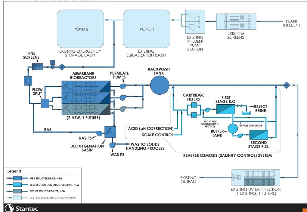
A two stage RO configuration is recommended for high water recovery (80% overall) is proposed. The reject stream from the first stream becomes the feed water from the second stage, as shown in **Figure 21**. In contrast to MBRs, there are no backwash mechanisms for RO systems, but they do require chemical cleaning.
