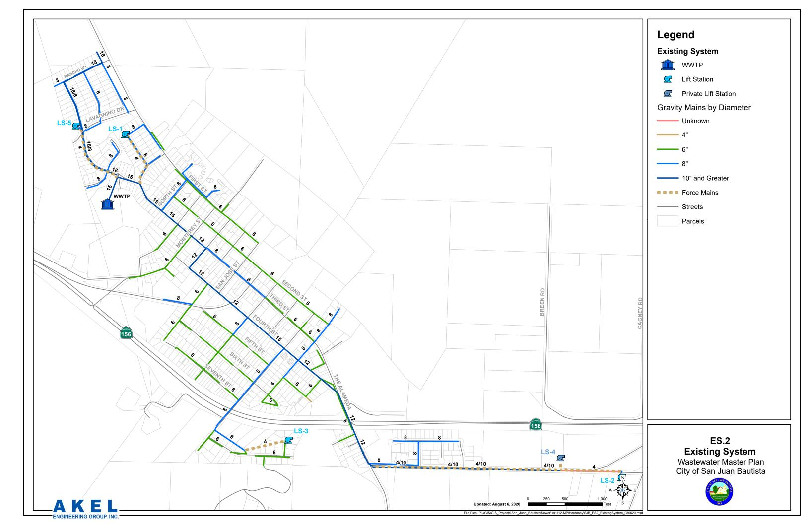
size. This figure provides a general color coding for the collection mains, as well as labeling the existing lift stations and WWTP.
